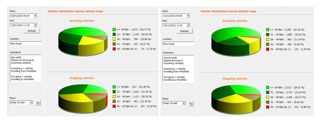
With the matrix switched to normal the percentage of vehicles traveling at less than 30mph has increased from 42.77 to 61.92%
