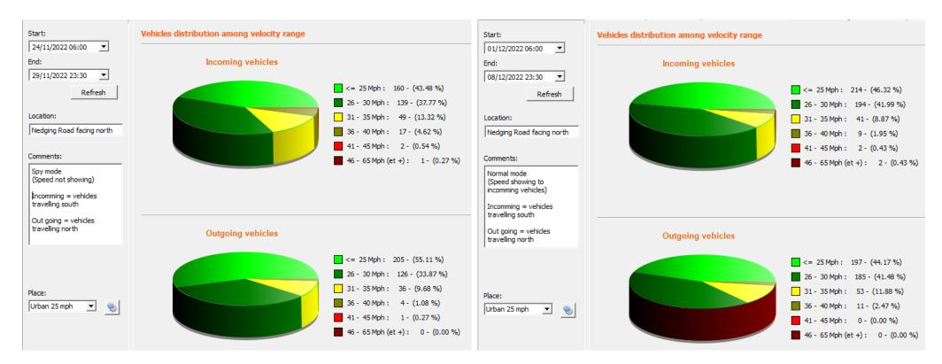
With the matrix switched to normal the percentage of vehicles traveling at less than 30mph has increased from 81.25 to 88.31%
