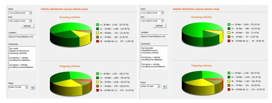
With the matrix switched to normal the percentage of vehicles traveling at less than 30mph has increased from 57.33 to 75.34%
